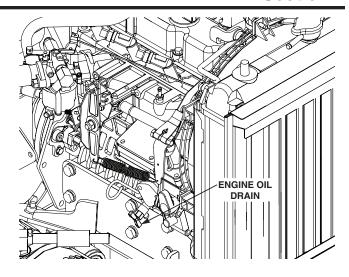
Figure 7-5. Drain Plug Location
